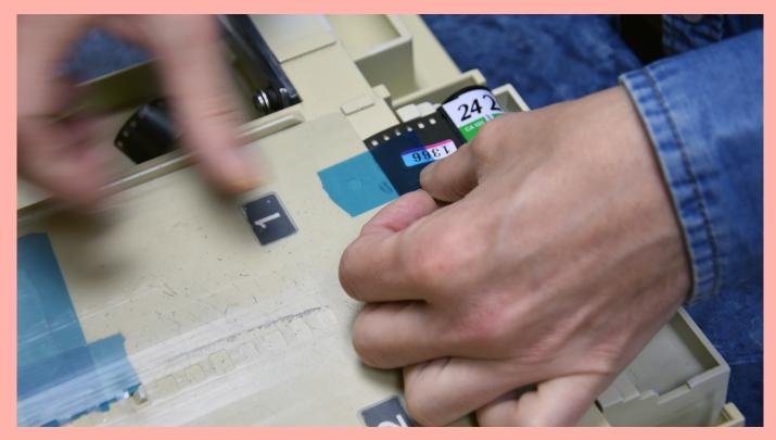
The plastic leader and the film cassette are then carefully loaded into the processing machine.
