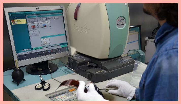
The negative strip is manually fed into the scanner and then mechanically drawn through the machine.
