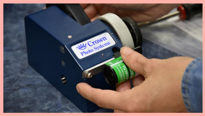
Once the film leader has been drawn out of the cassette, it is removed by slicing the end off.
