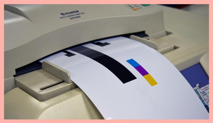
Our film has now passed through all of the chemistry and is being fed out of the end of the machine to dry.
