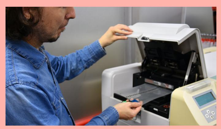
The internal mechanism of the processing machine draws the leader card through a series of rollers into different types of 'chemistry'.
